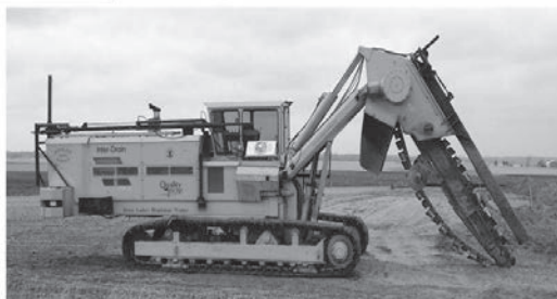
The Inter-Drain chain trencher. Four size choices, mechanical or hydraulic chain drive, vertical and offset available. Cummins, Volvo or Cat power.
