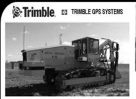
The Inter-Drain plow, three types, double link, single cantilever, or single link, each in three sizes. Cat, Cummins or Volvo power. Offset available.
