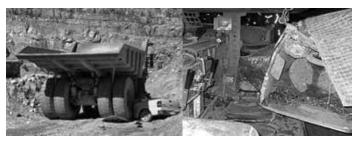
Roadway design and poor visibility at a nearly blind intersection were the root causes of a miner's death when his pickup was crushed by a haul truck A miner died when underground shuttle cars collided in an intersection. One shuttle care rammed through a ventilation curtain without stopping or warning.
