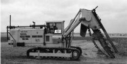
The Inter-Drain chain trencher. Four size choices, mechanical or hydraulic chain drive, vertical and offset available. Cummins, Volvo or Cat power.
