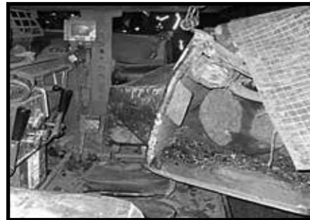
A miner died when underground shuttle cars collided in an intersection. One shuttle car rammed through a ventilation curtain without stopping or warning.
