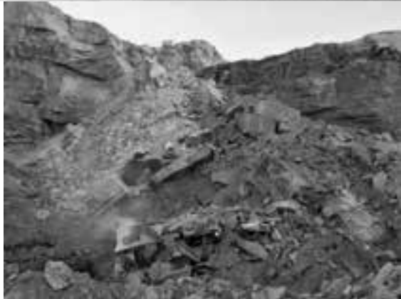
A miner was fatally injured at a surface coal mine while operating a front-end loader to remove shot rock near the base of a 63 ft. highwall.
