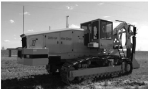
The Inter-Drain plow, three types, double link, single cantilever, or single link, each in three sizes. Cat, Cummins or Volvo power. Offset available.
