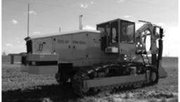
The Inter-Drain plow, three types, double link, single cantilever, or single link, each in three sizes. Cat, Cummins or Volvo power. Offset available.
