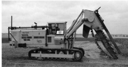
The Inter-Drain chain trencher. Four size choices, mechanical or hydraulic chain drive, vertical and offset available. Cummins, Volvo or Cat power.
